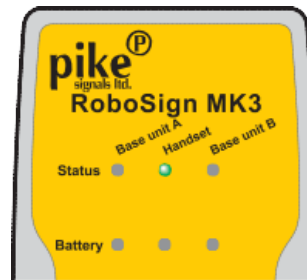
Remote control: The top centre green indicator should be on, the lower centre indicator should be off (see page 7)
