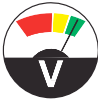
Base units: The volt metre needle should be in the green area. If not, the unit needs to be charged (see page 8)
