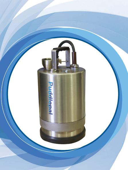
A versatile, portable, submersible, residue pump for clean water. The pump features the ability to pump down to 1mm, therefore ideal for removing water from flat surfaces such as floors and flat-roofs.
