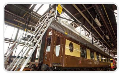
Spandeck used to gain close access for maintenance to the roof of the Famous Orient Express.
