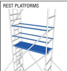
Rest platforms must be fitted every 2m and consist of a trap platform, and guardrails at 0.5m and 1m as shown. Remember to always close trapdoor immediately after climbing through. Nb. see safety note on back page.
