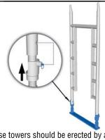
1. These towers should be erected by at least 2 competent persons. Fit an adjustable foot assembly into a walk through base frame ensuring that the spring loaded pins engage in the holes provided (1A).
