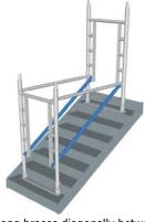
4. Fit two long braces diagonally between the bottom rungs of each frame. At this stage level the tower by adjusting the collars on the foot assemblies (see construction notes).
