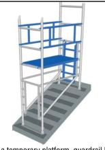
6. Now fit a temporary platform, guardrail brace frames & ladder as shown in steps 6, 7 & 8 opposite.
