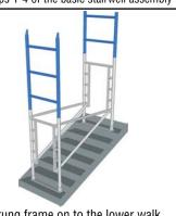
5. Fit a 3 rung frame on to the lower walk through base frame by locating onto head fitting with peg engaging into hold provided. Repeat the process at the other end using a 2 rung guardrail frame.
