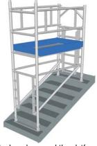
9. Fit the toeboards around the platform. Always remember to close the trapdoor immediately after climbing through.
