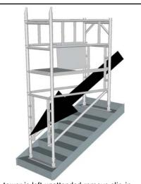
When tower is left unattended remove clip-in ladder & toeboard to allow emergency access through the tower. This can be further assisted by opening the trap door on the platform.
