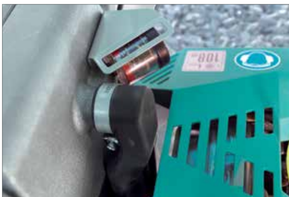
Voluminous but finely woven air filter with self-cleaning effect optionally equipped with a cyclone pre cleaner and a service indicator (gives up to five times longer service intervals)
